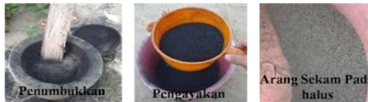
Figure 6. Process of refining husk charcoal
